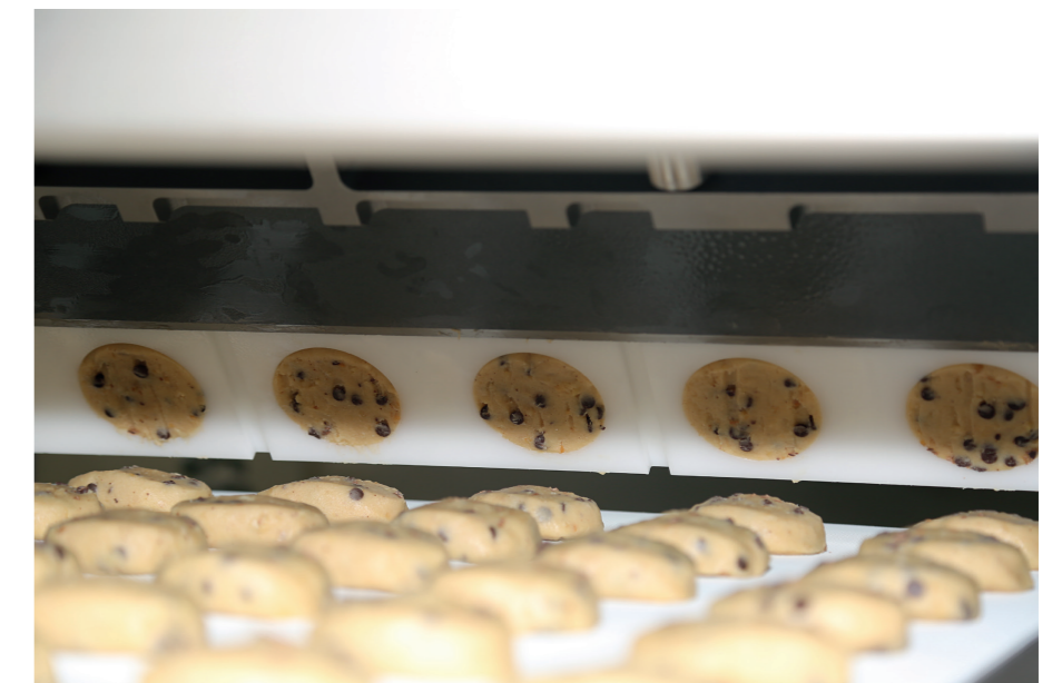
Multi-lane filling flow divider for portioning cookies
